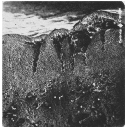
Figure 25 Severe degradation of microporous layer in poromeric degraded to 25% of its original tensile energy, after reconditioning the sample was flexed 20 000 times.
