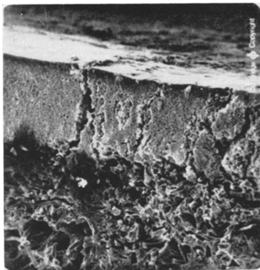
Figure 21 Sample of poromeric shoe upper with severe cracking in microporous layer due to degradation by sweat.
