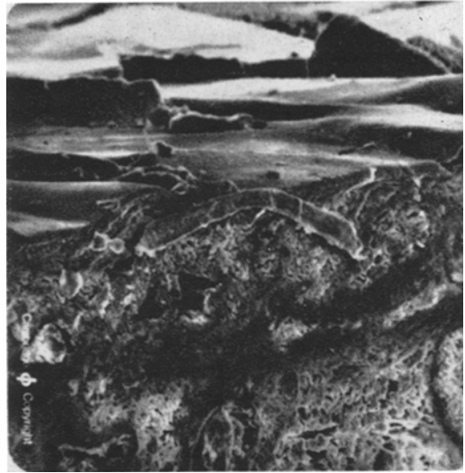
Figure 13 Cross-section of grained natural leather after 20 000 flexes.
