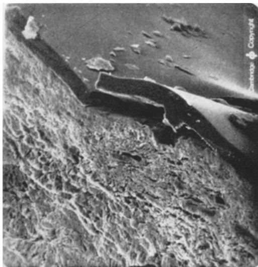
Figure 11 Delamination of polyurethane coating on a "wet look" leather.
