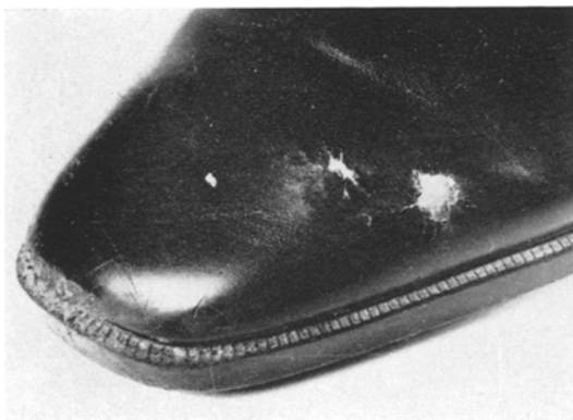
Figure 20 Poromeric shoe upper showing damaged microporous layer due to chemical degradation.
